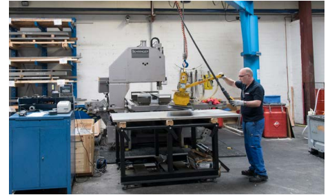
Kranbeschickung zu Säge Crane feeding to saw
