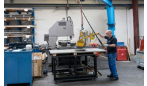
Kranbeschickung zu Säge Crane feeding to saw
